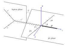
$\phi$  - the angle between lepton plane and jet plane
