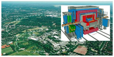
ZEUS: multipurpose, hermetic detector Total luminosity:  $\int \mathcal{L} \sim$  500 pb $^{-1}$  collected during HERA I + II running periods
