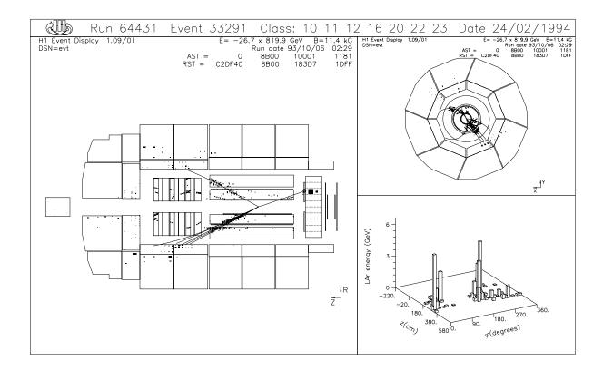
Figure 9.2: A H1 data event with the electron scattered in the BEMC calorimeter.
