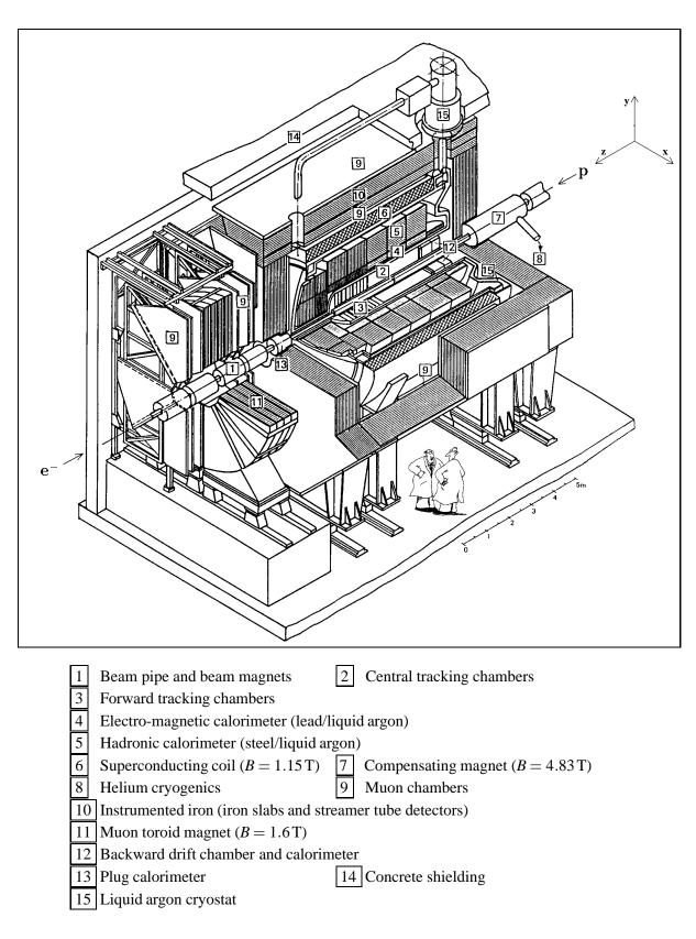
**Figure 3.3:** Schematic view of the H1 Detector. The H1 coordinate system is defined in the top right corner.
