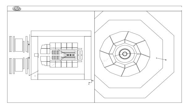
**Figure 4.1:** Schematic view of a typical event candidate for the process  $\gamma \rightarrow J/\psi p, J/\psi \rightarrow \mu\mu$ ; on the left hand side the side view of the H1 detector is shown and on the right hand side the radial view. Except for the two decay muons (one detected in the LAr calorimeter and in the instrumented iron, the other one only in the LAr calorimeter) the detector is empty; the invariant mass of the two muon system is 3.17 GeV.
