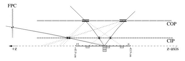
**Figure 3.12:** The *z*-vertex histogram in the *rz*-view for one  $\varphi$  sector is shown. Rays originating from genuine particles are indicated by full lines, while the dotted lines indicate the wrong combinations.
