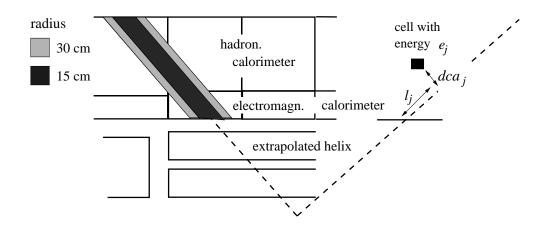
Figure 3.15: Schematic illustration of muon identification in the LAr calorimeter.
