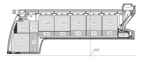
**Figure 3.8:** Side view of the upper part of the LAr calorimeter divided into electro-magnetic (dark shaded) and hadronic (light shaded) and inner forward (IF), outer forward (OF), forward barrel (FB), central barrel (CB) and backward barrel (BB) parts.
