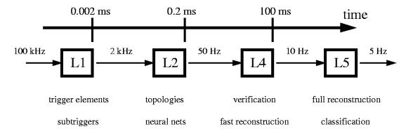
**Figure 3.10:** Trigger levels used during 1994 to 1997 data taking. Shown are typical rates and decision times for each level. The given keywords are explained in the text.
