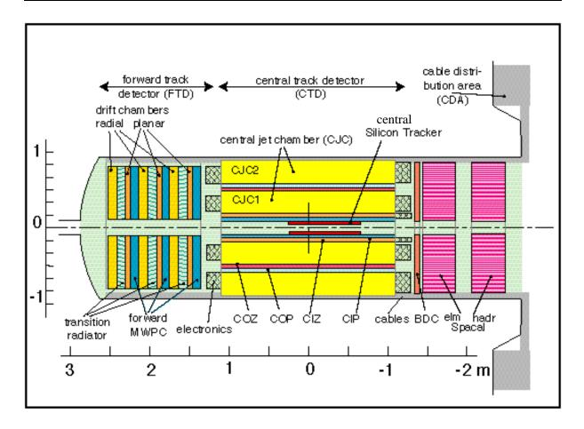
**Figure 3.4:** Schematic side view of the tracking system. In addition to the Forward Track Detector (FTD) and the Central Track Detector (CTD) the backward calorimeter SpaCal is also shown.
