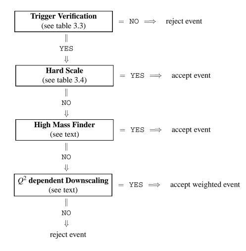
**Figure 3.13:** Schematic illustration of the L4 scheme including the steps which are important for this analysis. After the last step only weighted events are kept, where the weight reflects information about the number of similar rejected events.
