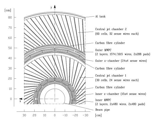
**Figure 3.5:** Schematic radial view of the Central Tracking Detector CTD, showing the Inner and Outer *z*-Drift Chambers, the Inner and Outer Multiwire Proportional Chambers and the two Jet Chambers in detail.
