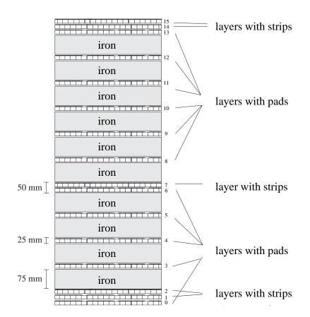
**Figure 3.7:** Schematic structure of the instrumented iron with its ten layers of streamer tubes equipped with strips or pads (3-12) in between ten layers of iron. On the inside and outside of the iron six additional strip layers (0-2,13-15) complement the track measurement. Layers 3, 4, 5, 8 and 12 are used for trigger purposes.
