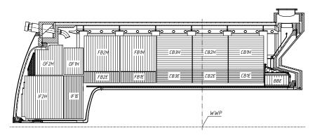
Figure 3.3: A side view of the Liquid Argon calorimeter.
