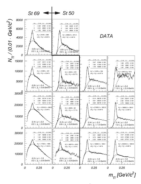
Figure 6.9:  $m_{\gamma\gamma}$  spectra (SpaCal) in intervals of the  $\pi^0$  transverse momentum and the  $\pi^0$  rapidity fitted by different functions. Table 6.1 gives the fit function referring to the number given in the plots. On the left of the marked line: mass spectra based on the minimum bias run of 1997 (St 69). On the right of the emphasised line: mass spectra based on data, selected by subtrigger 50 (St 50) in 1996.
