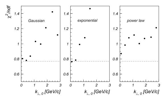
Figure 6.15:  $\chi^2/ndf$  as a function of the "primordial" intrinsic  $k_{\perp}$  assuming a Gaussian, exponential and power law  $k_{\perp}$  distribution. The  $\chi^2$  was obtained taking into account all data points from the double differential cross sections shown in Fig. 6.11 and 6.12.
