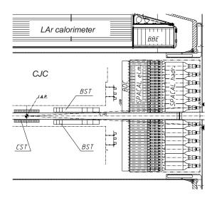
Figure 3.2: A side view of the backward region of the H1 detector.
