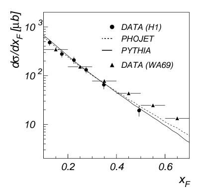
Figure 6.16: Inclusive  $\pi^0$  photoproduction cross section as a function of Feynman x. The curves are the predictions of the PHOJET (dashed) and PYTHIA (full) modells. The H1 data, at  $\sqrt{s_{\gamma p}} \approx 208$  GeV, as well as the MC model predictions, are obtained in the rapidity range -3.5 < y < -1.5. The data of the Omega Photon Collaboration (WA69), at  $\sqrt{s_{\gamma p}} \approx 12.3$  GeV, were derived as described in appendix C.
