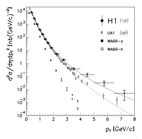
Figure 1.9: The inclusive double differential charged particle cross section  $d^2\sigma/d\eta dp_{\perp}^2$  as a function of the particles transverse momenta  $p_{\perp}$ , measured by the H1 Collaboration (full points) in the pseudo-rapidity range  $|\eta| < 1.5$ . The solid (dashed) line is the result of a power law fit (equation 1.29) to the H1 (UA1) data (see text).
