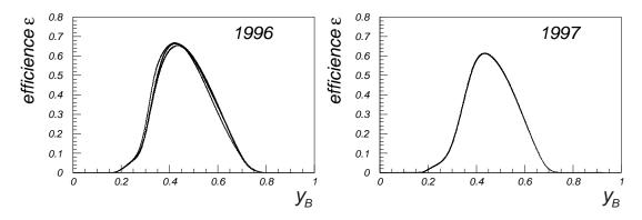
Figure 4.1: Run dependent efficiencies of the electron tagger as a function of  $y_B$  for the years 1996 and for the minimum bias data taking period of 1997.
