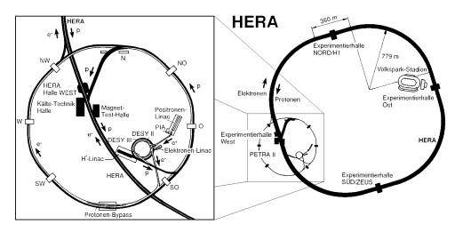
Figure 2.1: Schematic overview of the HERA accelerator complex
