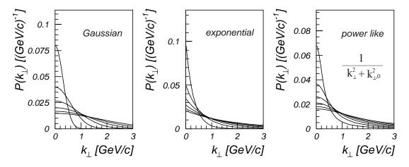
Figure 1.8: Three assumptions on the primordial  $k_{\perp}$  distributions of the photon remnant: a Gaussian, an exponential and a power law distribution. The width of the distributions increases from 0.3 GeV/c to 1.8 GeV/c in steps of 0.3 GeV/c.
