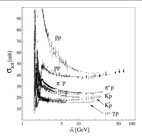
Figure 1.3: Total cross section for various particle reactions as a function of the CM energy. The photon-proton cross sections have been multiplied by a factor of  $\frac{1}{\alpha_{em}}$ .
