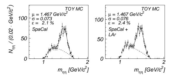
Figure 8.5:  $TOY\ MC$ : Two- $\eta$  spectra as seen in the SpaCal (left side) and as seen in the SpaCal and LAr calorimeters together (right side). Only the  $f_0(1500)$  meson, scattered into the backward region of the H1 calorimeter, was generated by the TOY MC. The reconstruction efficiencies  $\epsilon$  for the  $f_0(1500)$  reconstruction are shown in the plots.
