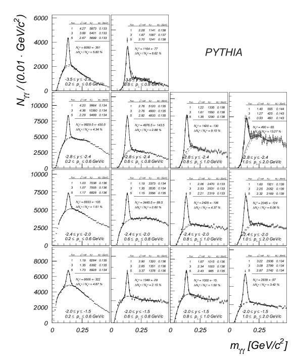
Figure 6.10: MC PYTHIA:  $m_{\gamma\gamma}$  spectra (SpaCal) in intervals of the  $\pi^0$  transverse momentum and in intervals of the  $\pi^0$  rapidity fitted by different functions. Table 6.1 gives the fit function referring to the number given in the plots.
