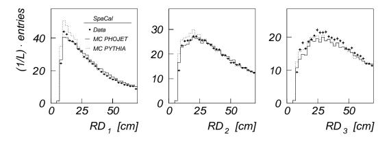
Figure 5.7: SpaCal: Comparison of the radial distribution of the three most energetic clusters in data (points) and the MC models PHOJET (full line) and PYTHIA (dotted line).
