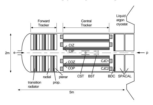
Figure 3.4: A side view of the H1 tracking system.
