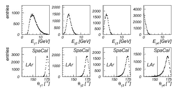
Figure 8.9: TOY MC: Energy and polar angle distributions of the four decay photons of the exclusively produced  $f_2(1270)$  as seen in the lab system. The line indicates the polar angular acceptance regions of the SpaCal and LAr calorimeter, respectively.
