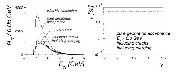
Figure 6.4: Left side: Comparison of the energy of all two-photon combinations between the TOY (see text) and the full detector simulation. The values of the z-coordinate of the LAr calorimeter were restricted to the range -150 < z < 200 cm. Right side: The  $\pi^0$  reconstruction efficiency (LAr) for the conditions listed in the legend of the plot.
