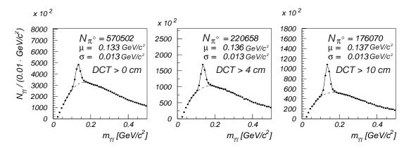
Figure 5.13: SpaCal:  $m_{\gamma\gamma}$  distributions for different cuts on the distance of the cluster center to the closest BDC track (DCT = Distance of Cluster center to closest Track).
