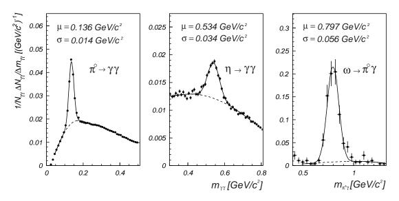
Figure 5.2: The inclusive  $\pi^0$ ,  $\eta$  and the exclusive  $\omega$  signals as seen in the SpaCal after applying the energy scale correction with the help of the  $\pi^0$  mass.
