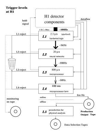
Figure 3.6: The trigger levels at H1.
