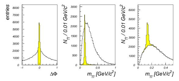
Figure 6.5: Left side: the difference  $f_{gen.} - f_{det.}$  for the  $\pi^0 s$  found in the SpaCal. Middle: two-photon mass spectra with photon candidates having a strong correlation to generated photons (grey coloured) and two-photon mass spectrum were no correlated photon on generator level could be found. Right side: the sum of the mass spectra shown in the middle plot.
