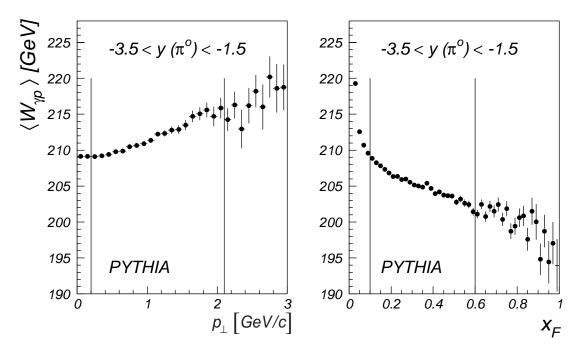
Figure 6.18: PYTHIA:  $\langle W_{\gamma p} \rangle$  as a function of the  $\pi^0$  transverse momentum and as a function of  $x_F$ . The region within the two vertical lines of each plot mark the range covered by this measurement.
