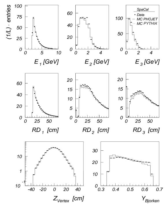
Figure 5.9: SpaCal: Comparison of data selected by subtrigger 50 and the reweighted MC models PHOJET (full line) and PYTHIA (dotted line).  $E_1$  -  $E_3$  = Energy of the first three most energetic clusters,  $RD_1$  -  $RD_3$  the corresponding radial distance of the cluster center from the beam line. The z-vertex and the  $y_B$  distribution.
