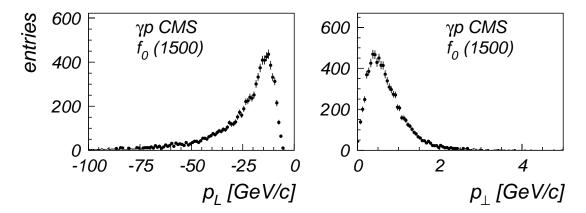
Figure 8.2: Longitudinal (left side) and transverse (right side) momenta of the  $f_0(1500)$  meson in  $\gamma p$  CMS, used in the TOY MC.
