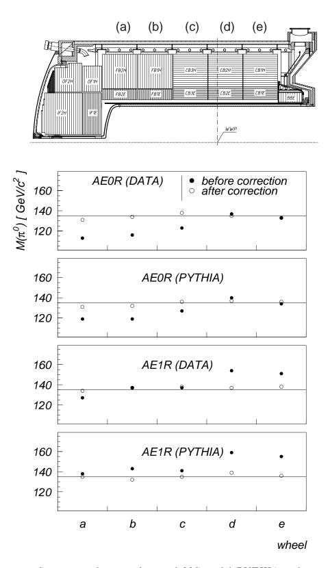
Figure 5.16: Comparison between data and MC model PYTHIA with respect to the  $\pi^0$  mass reconstructed from photons flying into the same LAr wheel. The full points are the values of the  $\pi^0$  mass before the mass correction and the open points are the values of the  $\pi^0$  mass after the mass correction.
