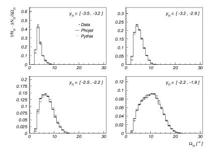
Figure 6.7: Opening angle  $\Omega_{\gamma\gamma}$  of all possible two-cluster combinations in the mass band of the  $\pi^0$  (0.1 <  $m_{\gamma\gamma}$ < 0.17 GeV/ $c^2$ ) in intervals of the rapidity of the cluster pairs (SpaCal).
