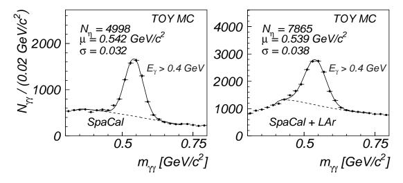
Figure 8.4: TOY MC: The two-photon distribution of the decay  $f_0(1500) \to \eta \eta \to \gamma \gamma \gamma \gamma$  as reconstructed in the SpaCal (left side) and as reconstructed in both, the SpaCal and LAr calorimeters (right side).
