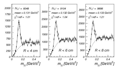
Figure 5.19: LAr:  $m_{\gamma\gamma}$  distributions with different cuts on the cluster radius R.
