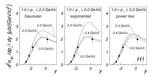
Figure 6.14: The  $\pi^0$  cross section as a function of the  $\pi^0$  rapidity y for the  $p_{\perp}$  range indicated in the figure. The curves are predictions of PYTHIA, labelled with the corresponding  $k_{\perp,0}$  values, as described in the text.
