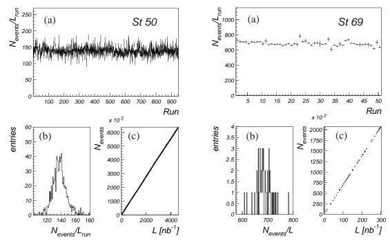
Figure 4.3: The number of events in the plots a,b and c fulfil the selection cuts listed in table 4.1 for subtrigger 50 and 69 respectively. (a) Number of events over the run luminosity as a function of the run number. (b) Number of events per run luminosity. (c) Number of selected events as a function of the integrated luminosity.
