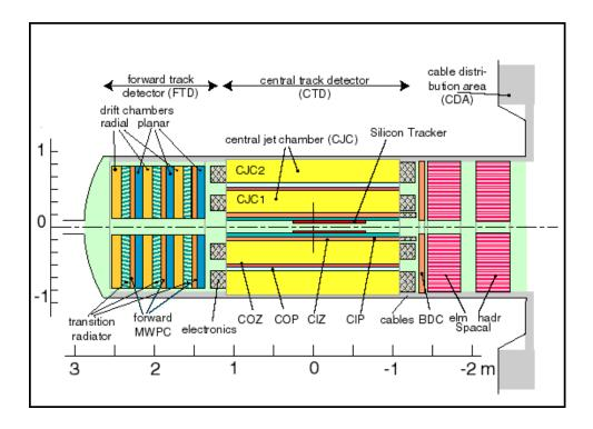
Figure 2.3: A longitudinal view of the H1 tracking system.
