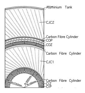
Figure 2.4: A section through the  $r - \phi$  plane of the central tracking detector.
