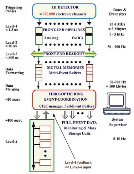
Fig. 3. H1 data acquisition system scheme
