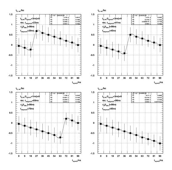
Figure 5.11.: Simulated dependence of the mean  $t_{0,rel.}$  on  $t_{synch}$  for a uniformly distributed detection time  $t_{det}$  of width  $\sigma_0(t_{det}) = 90$ ns and four different phases of resynchronisation  $t_{resynch}$ . In addition, the reconstructed value of  $t_{resynch}$  is given. Errors give rms of mean  $t_{0,rel}$ .
