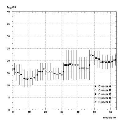
Figure 5.2.: Times of Flight  $t_{\text{flight}}$  for each module (trigger layers only)
