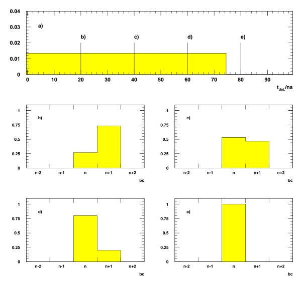
Figure 5.1.: Synchronisation of the initial digital wire signals a) Normalised uniform distribution  $p_{det}(t_{det}(t_0 = 0))$  of the detection time  $t_{det}$  of width 75ns b)-e) Timeslice distributions resulting from different  $t_{synch}$  indicated in a)
