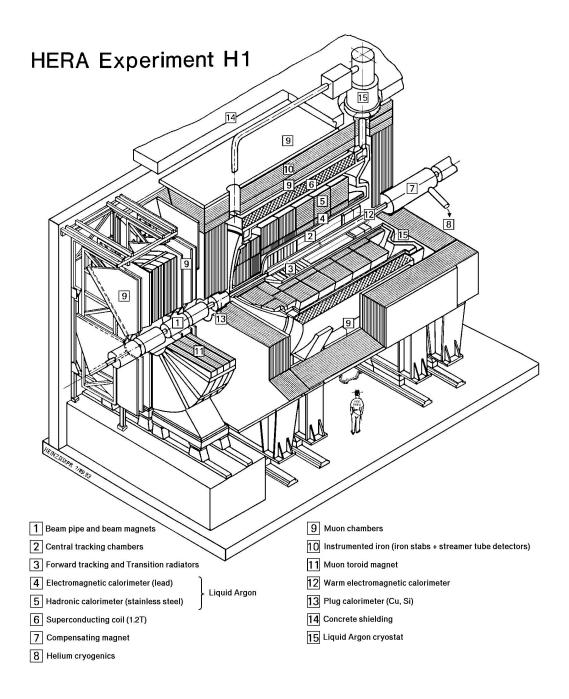
Figure 1.2.: The H1 Detector at HERA
