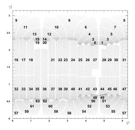
Figure 1.6.: Coverage of the  $\vartheta - \varphi$ -Plane by the (iron) modules of the Central- $\mu$ -Detector
