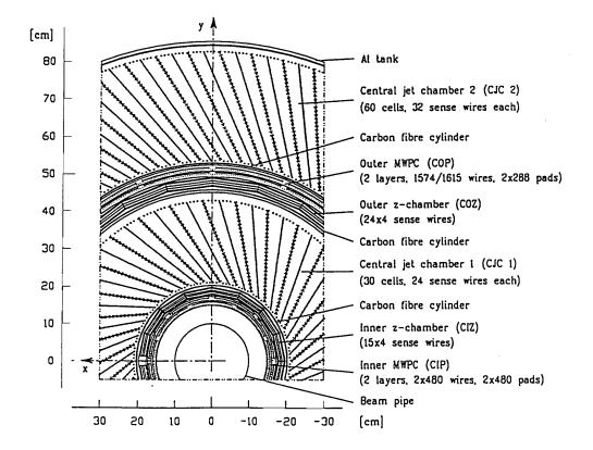
Figure 1.10.: A radial cut through the central tracking detectors perpendicular to the beam.
