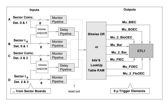
Figure 3.6.: Scheme of the functionality of General Purpose Trigger Pipe Board
