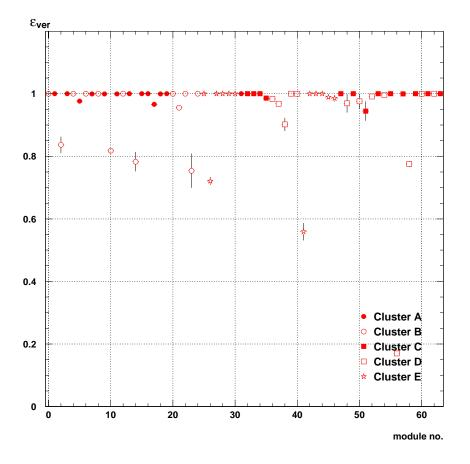
Figure 8.2.: Verification efficiency of L2/L3 data (layer coincidence bits) from combined cosmic and proton beam halo calibration data
