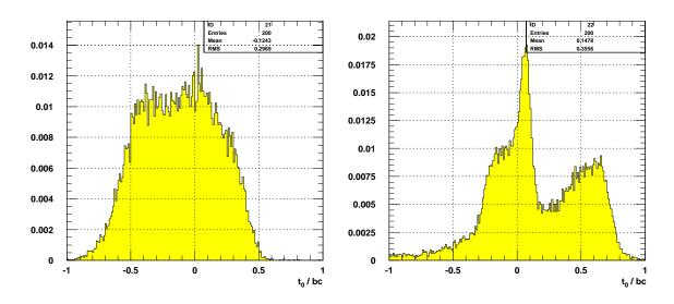
Figure 5.15.: Normalised distributions of the  $t_0$  reconstructed in the CJC for CIP-4 cosmic data (left) and in the Forward  $\mu$  Detector for beam halo data (right)
