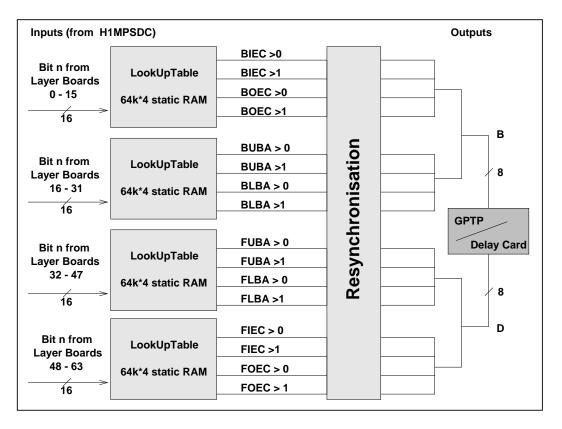
Figure 3.5.: Scheme of the Sector Board functionality
