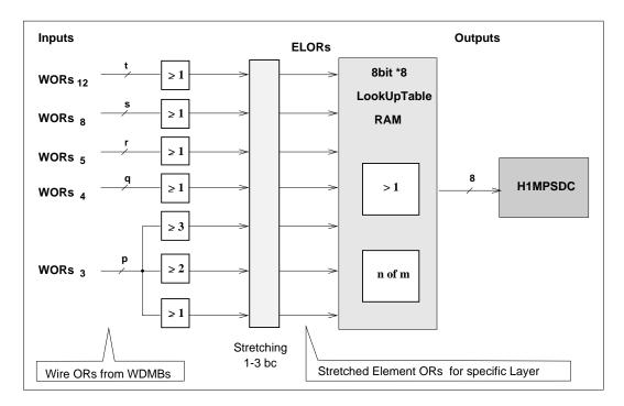
Figure 3.4.: Scheme of the Layer Board functionality (letters {p,q,r,s,t} mean number of elements connected to the input port)
