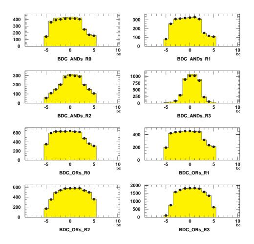
Figure 6.3.: Trigger verification type B, based on readout data of beam halo events triggered by dedicated subtriggers (20 or 21): number of events with active TE vs. bunch-crossing (dots: real TE data, grey: triggers simulated from readout data).
