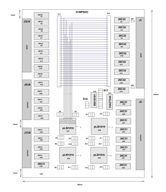
Figure E.1.: Component side view of the H1MPSDC. Top left : input connectors J3–J6 for usage in a standard VME crate (6HU), bottom left output connectors, top right: J1, input connector during usage in the SB crate Jumper SP1, defining the power source line from J1 has to be changed to SP2 during usage in a standard VME crate, bottom right: connectors J7–J10, providing the PLCC output.
