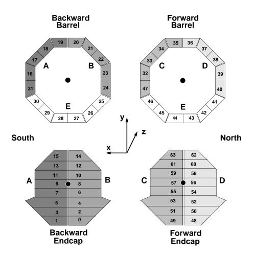
Figure 1.5.: Division of the Central– $\mu$ –Detector into 64 modules and their assignment to hardware clusters A–E
