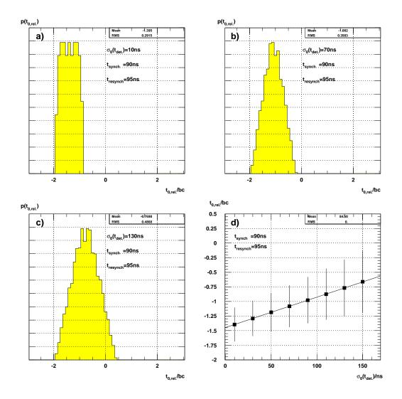
Figure 5.7.: a)-c): Simulated distributions of  $t_{0,rel}$  for three different values of  $\sigma_0(t_{det})$  and constant  $t_{synch}$  and  $t_{resynch}$ . Figure d) shows the mean  $t_{0,rel}$  vs  $\sigma_0(t_{det})$  for  $10ns \leq \sigma_0(t_{det}) \leq 150ns$ .
