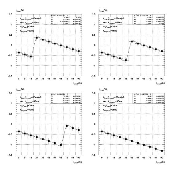
Figure 5.9.: Simulated dependence of the mean  $t_{0,rel.}$  on  $t_{synch}$  for a uniformly distributed detection time  $t_{det}$  of width  $\sigma_0(t_{det}) = 30$  ns and four different phases of resynchronisation  $t_{resynch}$ . In addition, the reconstructed value of  $t_{resynch}$  is given. Errors give rms of mean  $t_{0,rel}$ .
