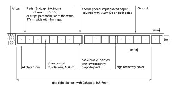
Figure 1.3.: Cut through a Central- $\mu$ -LST element perpendicular to the wires
