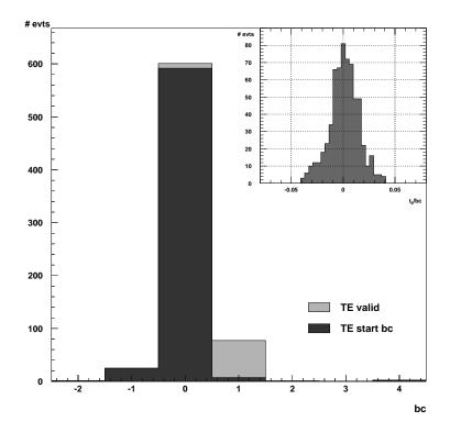
Figure 4.5.: Usage of the coincidence and the  $t_0$  signal for the TE: Distributions of all and first timeslices in which TE was active (TE BIEC>0, for a layer coincidences in only one module of the sector Luminosity run 181249). The insert shows the distribution of the  $t_0$  reconstructed from CJC data.
