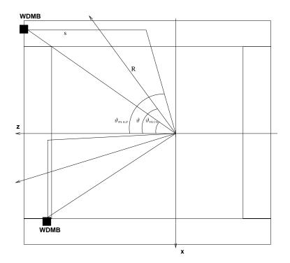
Figure 5.3.: The correlation of the time of flight  $t_{\text{flight}}$  and the transmission time  $t_{\text{trans}}$  (top view of the Central- $\mu$ -Detector ).
