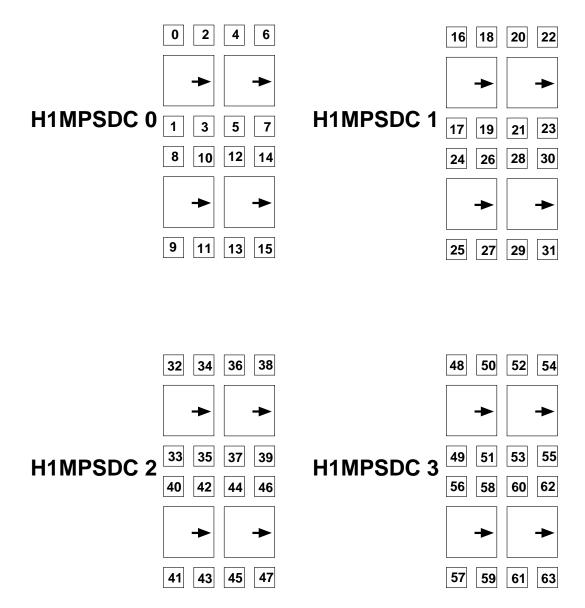
Figure E.2.: Assignment of the LB to the three–bit switches defining the delay on the H1MPSDC
