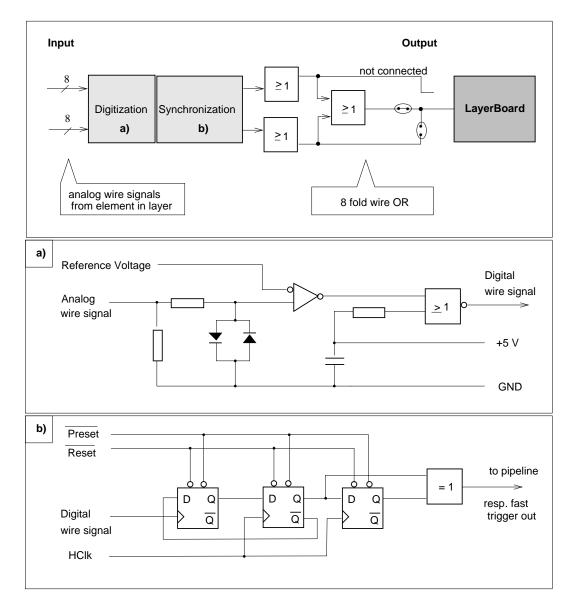
Figure 3.3.: Scheme of the WDMB functionality
