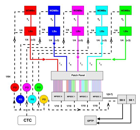
Figure 5.6.: The distribution of the HClk to the Central- $\mu$ -Trigger System from the CTC to the WDMBs and the data flow back to the GPTP. Expressions like 1/n(<m) indicate the possibility to delay the respective signal in steps of  $\frac{1}{n}$  bc in a range up to m bc
