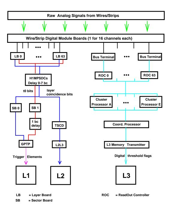
Figure 3.1.: The trigger data flow from the chambers to L1, L2, L3
