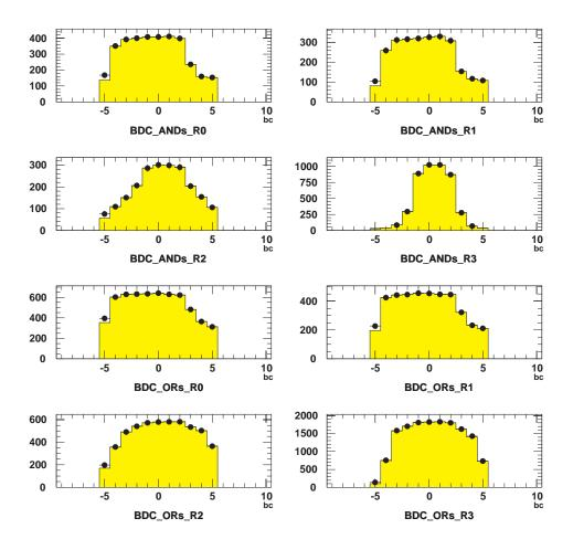
Figure 6.2.: Trigger verification type A, based on TE data (TEL1) of beam halo events triggered by the dedicated subtriggers (20 or 21): number of events with active TE vs. bunch-crossing (dots: real TE data, grey: triggers simulated from readout data).
