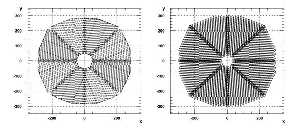
Figure 1.8.: Geometry of a  $\varphi$ - and a  $\vartheta$ -double-layer of the Forward-Muon-Spectrometer
