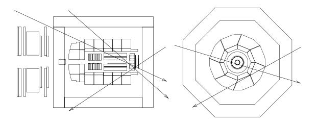
Figure 6.4.: Topologies triggered with the cosmic calibration setup for the BDC and the SpaCal (left) and for the Tail Catcher Calorimeter (right)
