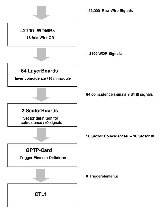
Figure 3.2.: The reduction of the L1 trigger data from the Central– $\mu$ –Detector
