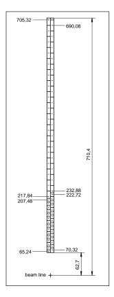
Figure 1.12.: Cut through a BDC double layer octant perpendicular to the wires
