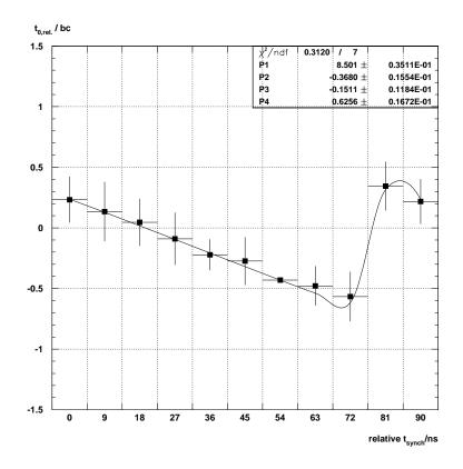
Figure 5.19.: Dependence of the mean  $t_{0,rel}$  on  $t_{synch}$  for triggers from module 28 in calibration runs.  $t_{synch}$  here has to be understood as  $t_{synch} + const.$ , with an unknown constant
