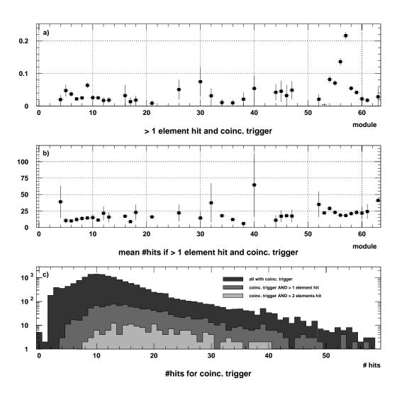
Figure 4.1.: a) Fraction of events with more than 1 element hit if layer coincidence condition fulfilled b) mean number of hits for events in a) c) number of hits for the number of hit elements > 0, > 1, > 2
