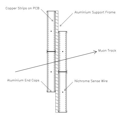
Figure 1.9.: Cut through cells in a double layer of the H1–Forward–Muon–Spectrometer
