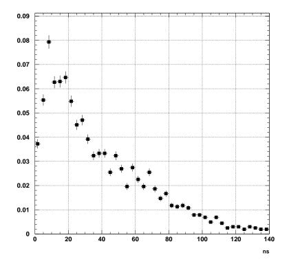
Figure 5.5.: Normalised drift time distribution  $p_{drift}(t_{drift})$  in an LST, with the threecomponent gas and a high voltage of 4.5kV without a magnetic field (from [35])
