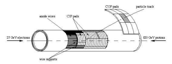
Figure 1.11.: The Central Inner and Outer Proportional Chambers of H1
