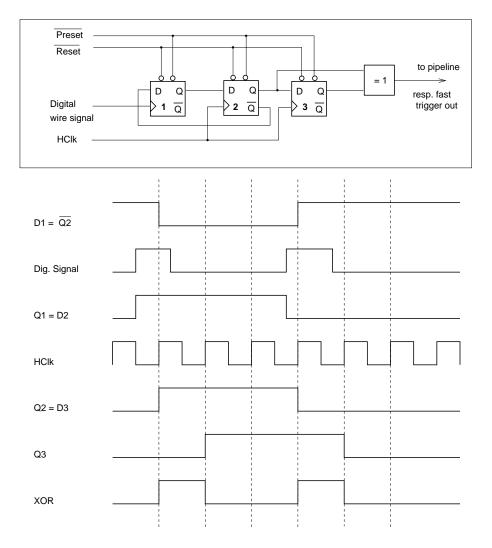
Figure D.1.: The synchronisation of the digitised wire (strip) signals on the WDMB
