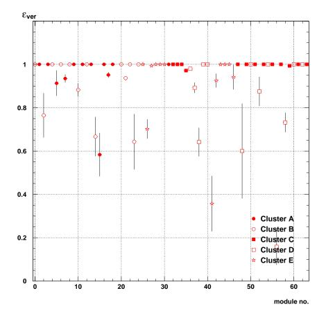
Figure 8.1.: Verification efficiency of L1 triggers from combined cosmic and proton beam halo calibration data
