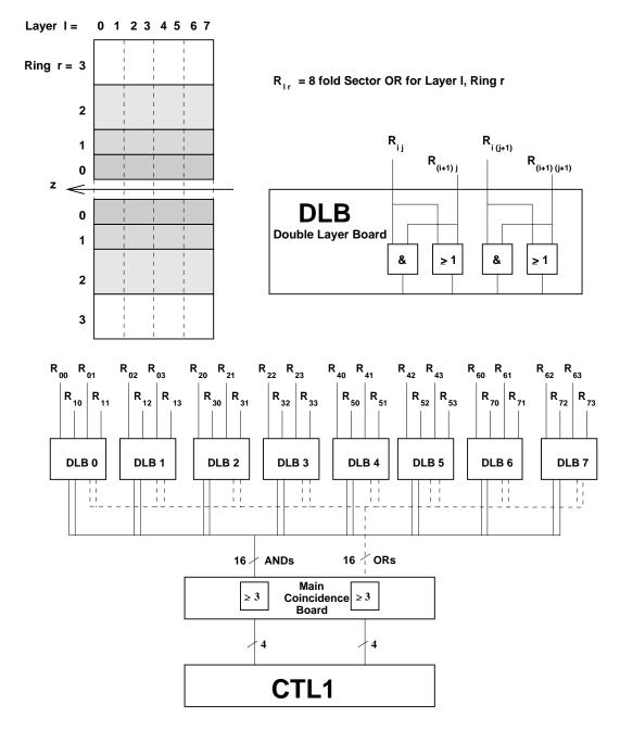
Figure 6.1.: Flow of the BDC trigger data from front end (WDMB) to CTL1
