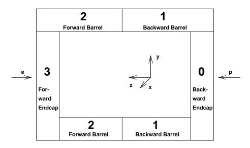
Figure 1.4.: Division of the Central- $\mu$ -Detector in  $\mu$ -subdetectors
