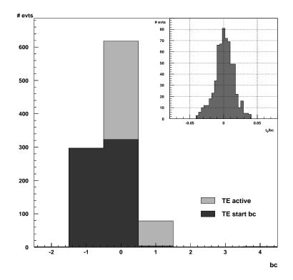
Figure 4.3.: Exclusive usage of the coincidence signal for the TE: Distributions of all and first timeslices in which TE was active (TE Mu\_BIEC>0, for a layer coincidences in only one module of the sector, luminosity run 181249). The insert shows the distribution of the  $t_0$  reconstructed from CJC data.
