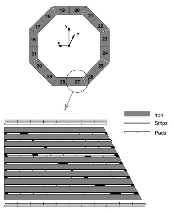
Figure 1.7.: Cut through a module in the Barrel, perpendicular to the wires, showing the different instrumentation of the layers
