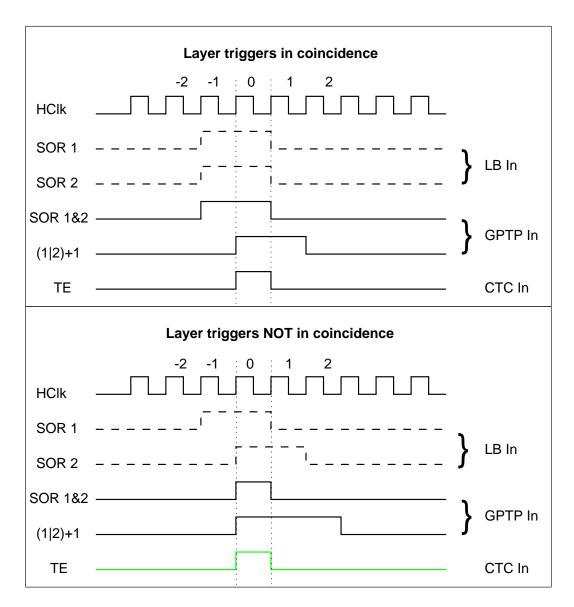
Figure 4.4.: Combination of the sector coincidence and  $t_0$  signal to the final  $\mu$ -TE.
