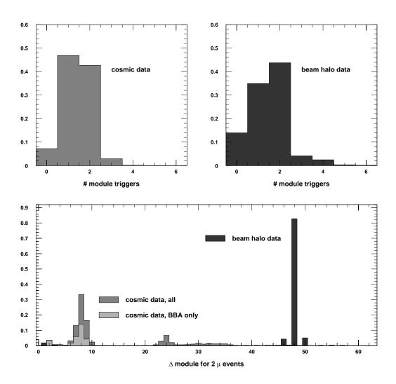
Figure 7.1.: Top left:distribution of number of module triggers in cosmic data top right: distribution of number of module triggers in beam halo data, bottom: difference of module numbers for muons events from cosmic radiation and the proton beam halo.
