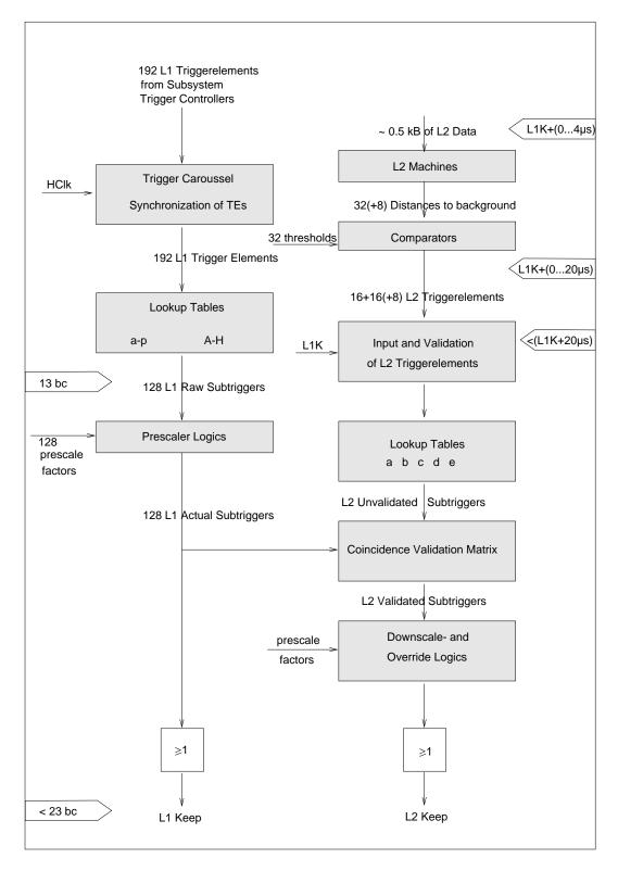
Figure 2.1.: The trigger data flow and relevant times on L1 and L2
