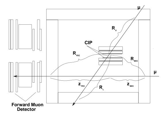
Figure 5.18.: Times of Flight to be considered in the calculation of the relative  $t_0$  from cosmic and beam halo calibration muons
