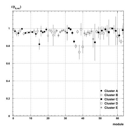
Figure 5.22.: The efficiency  $\varepsilon(t_{0,rel})$  at  $t_{0,rel} = 0$  for each single module derived from cosmic and beam halo calibration runs.
