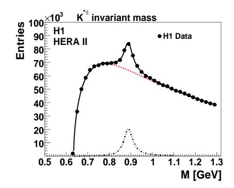
**Figure 7.11:** Invariant mass spectra of  $K_S^0 \pi^{\pm}$  combinations after application of the all cuts mentioned in details in the text. The distribution is fitted with a relativistic Breit-Wigner function (solid line) and a background function (dashed line). The signal is shown with dash-dotted lines.
