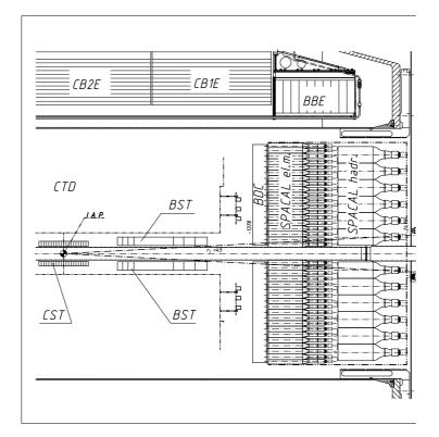
Figure 4.9: The location of SPACAL in the H1 detector.
