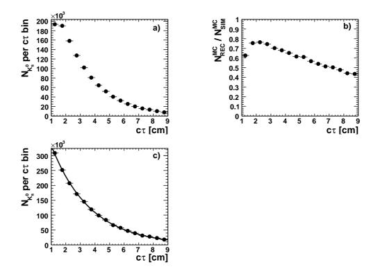
**Figure 7.6:** The lifetime of  $K_S^0$  candidates: a) uncorrected data, b) the ratio of simulated to reconstructed DJANGO events, c) corrected lifetime which is the resultant of application of ratio to the uncorrected data. The solid line represents the result of an exponential fit.
