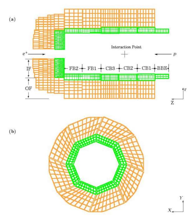
**Figure 4.8:** The LAr Calorimeter. a) the structure of wheels, b) the octant structure of wheels.
