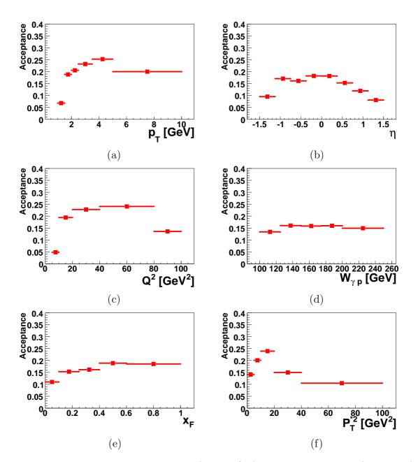
Figure 8.2: The acceptance correction factors  $\mathcal{A}$  of the H1 detector as a function of all measured quantities of the  $K^{*\pm}$  cross section: (a) the transverse momentum  $p_T$ , (b) the pseudorapidity  $\eta$ , (c) the four momentum squared  $Q^2$ , (d) the centre-of-mass energy of the hadronic final state  $W_{\gamma p}$ , (e) the Feynman variable  $x_F$ , and (f) the squared transverse momentum of the  $K^{*\pm}$  meson in the photon proton rest frame,  $P_T^{*2}$ .
