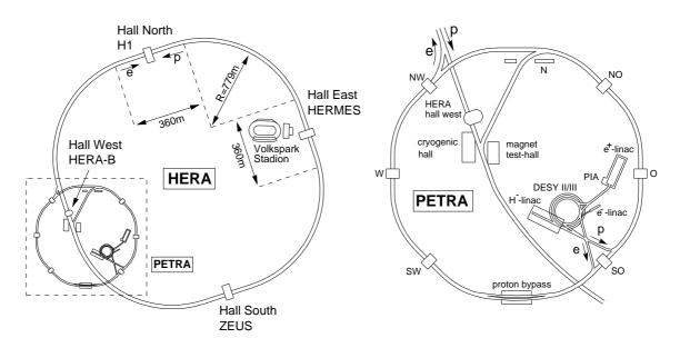
Figure 4.1: Layout of HERA collider, and its injection and its pre-accelerators.
