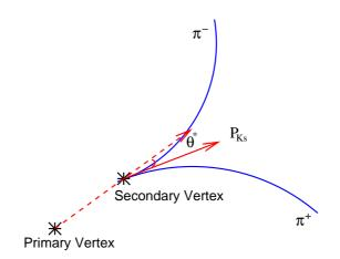
**Figure 7.1:** A schematic view of an event with a  $K_S^0$  decay. The  $K_S^0$  is produced at the point represented *primary vertex* and travels some distance before it decays at which the point represented as *secondary vertex*. The  $K_S^0$  decays in two pions which can be detectable. The dashed line from primary to secondary vertex shows the undetectable trajectory of the  $K_S^0$ .
