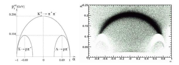
Figure 7.3: Armenteros-Podolanski plot shown in idealised form (left panel), and as measured in the present analysis (right panel).
