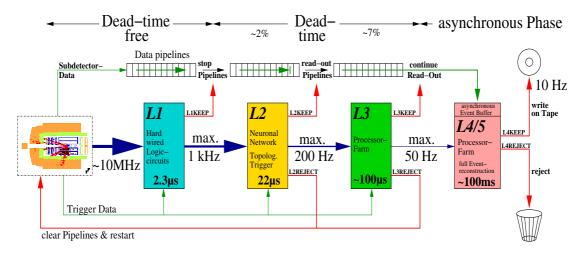
Figure 4.12: An illustration of the data flow through the H1 trigger system.
