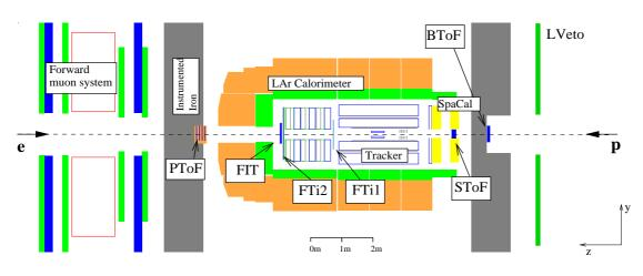
Figure 4.11: The Time-of-Flight system.
