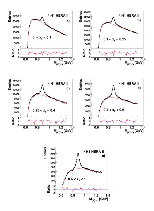
Figure 7.14: Invariant mass spectra of  $K_S^0 \pi^{\pm}$  combinations in intervals of scaled longitudinal momentum  $x_F$ ; a)  $0. < x_F < 0.1$ , b)  $0.1 < x_F < 0.25$ , c)  $0.25 < x_F < 0.4$ , d)  $0.4 < x_F < 0.6$  and e)  $0.6 < x_F < 1$ . The distribution is fitted with a relativistic Breit-Wigner function (black line) and a background function (red line). On the bottom of each figure the ratio distribution, Ratio =  $(N^{DATA} - N^{FIT})/\sqrt{N^{DATA}}$ , is shown.
