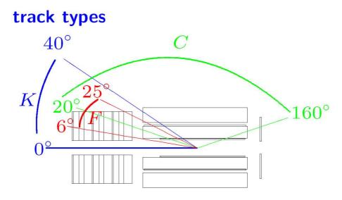
**Figure 6.5:** Angular ranges of the various track types: central  $(20^{\circ} < \theta < 160^{\circ})$ , forward  $(6^{\circ} < \theta < 25^{\circ})$  and combined  $(0^{\circ} < \theta < 40^{\circ})$ .
