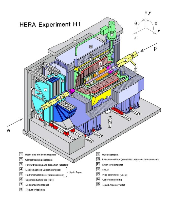
Figure 4.4: The H1 detector with its major components [117].
