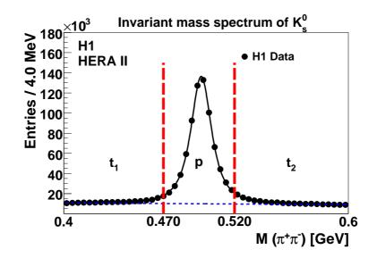
**Figure 8.6:** The terms which are used for the calculation of the ratio  $R = \frac{p}{t_1 + p + t_2}$ .
