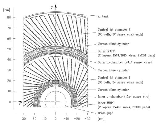
Figure 4.6: A radial view of the central tracking.
