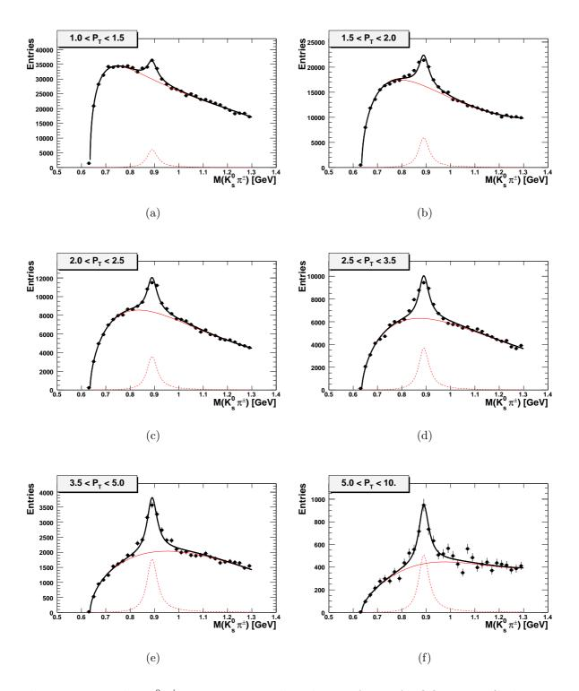
Figure 7.13: The  $K_S^0 \pi^{\pm}$  invariant mass distribution for DJANGO Monte Carlo simulation in intervals of transverse momentum  $p_T$ ; (a)  $1 < p_T < 1.5$ , (b)  $1.5 < p_T < 2$ , (c)  $2 < p_T < 2.5$ , (d)  $2.5 < p_T < 3.5$ , (e)  $3.5 < p_T < 5$  GeV and (f)  $5 < p_T < 10$  GeV. The distribution is fitted with a relativistic Breit-Wigner function (black line) and a background function (red line). The signal is shown with dashed lines.
