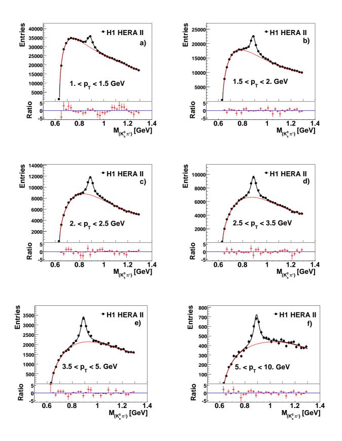
Figure 7.12: Invariant mass spectra of  $K_S^0 \pi^{\pm}$  combinations in intervals of transverse momentum  $p_T$ ; a)  $1 < p_T < 1.5$ , b)  $1.5 < p_T < 2$ , c)  $2 < p_T < 2.5$ , d)  $2.5 < p_T < 3.5$ , e)  $3.5 < p_T < 5$  and f)  $5 < p_T < 10$  GeV. The distribution is fitted with a relativistic Breit-Wigner function (black line) and a background function (red line). On the bottom of each figure the ratio distribution, Ratio =  $(N^{DATA} - N^{FIT})/\sqrt{N^{DATA}}$ , is shown.
