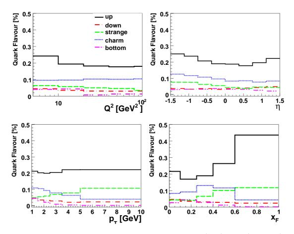
Figure 9.7: The relative fractions of the different quarks (up (full line), down (dashdotted line), strange (dash line), charm (dotted line) and bottom (dash-double-dotted line)) are shown. contributing in the hard interaction to the production of  $K^{*\pm}$  in the visible range. The fractions are shown as a function of  $Q^2$ ,  $\eta$ ,  $p_T$  and  $x_F$ .
