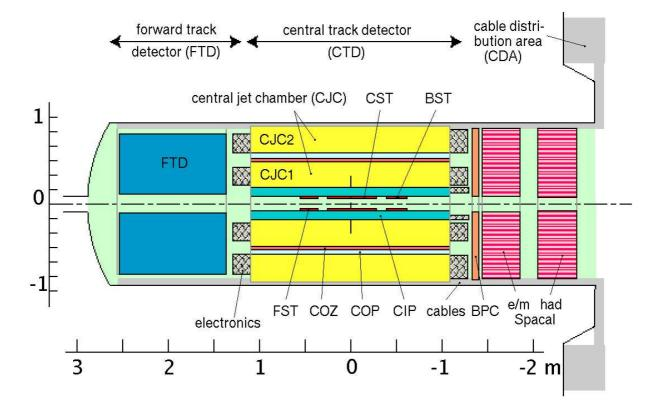
**Figure 4.5:** A longitudinal view of the H1 tracking system including the central and forward tracking detectors.
