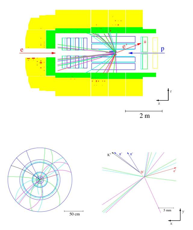
Figure 5.12: Event display of a dijet event with a reconstructed D\* meson. The electron is scattered into the backward calorimeter tagging this as a DIS event, the proton remnant traverses the forward tracker. In the upper schematic the detector is shown in the rz plane. Below the central tracking system is shown in the  $r\phi$  plane. On the right hand side a detailed view of the reconstructed tracks around the primary event vertex is given.
