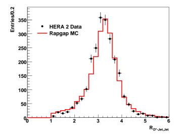
Figure 5.1: Distance in  $\eta$ - $\phi$  between the identified  $D^*$ -jet and the highest-remaining- $p_t$  jet for HERA 2 signal events compared to the Monte Carlo simulation. The distinct peak around the value  $\pi$  visualises the back-to-back topology in  $\phi$ .
