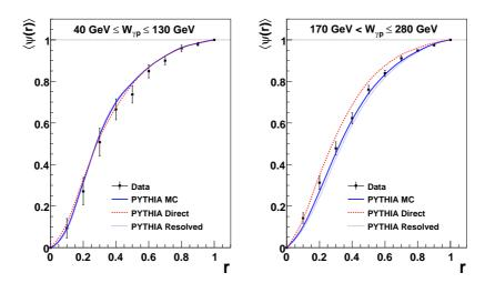
Figure 6.18: Mean integrated jet shape  $\langle \psi(r) \rangle$  in photoproduction at detector level as function of the cone radius r for two different regions of  $W_{\gamma p}$ . Pythia charm Monte Carlo prediction is shown together with separate direct and resolved expectations. Only statistical errors of the data are shown. The statistical errors of the Monte Carlo simulation are negligible.
