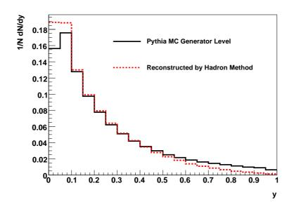
Figure 4.3: Distribution of the inelasticity y in photoproduction on generator level and reconstructed by the hadron method. Due to the Etag acceptances the y-range is limited to 0.05 < y < 0.65. Within these boundaries the reconstruction method performs reasonably well.
