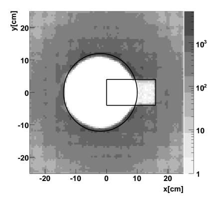
Figure 5.10: Inner SpaCal hitmap showing the distribution of the reconstructed impact positions of the scattered electrons in the backward calorimeter (HERA 2 data). No cuts are applied. The radial and box cuts are shown.
