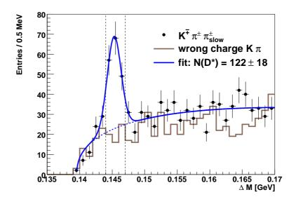
Figure 5.6: Distribution of the difference  $\Delta m$  between the invariant mass of the D<sup>\*</sup> candidate and the D<sup>0</sup> candidate after photoproduction jet selection for the ET44 sample.
