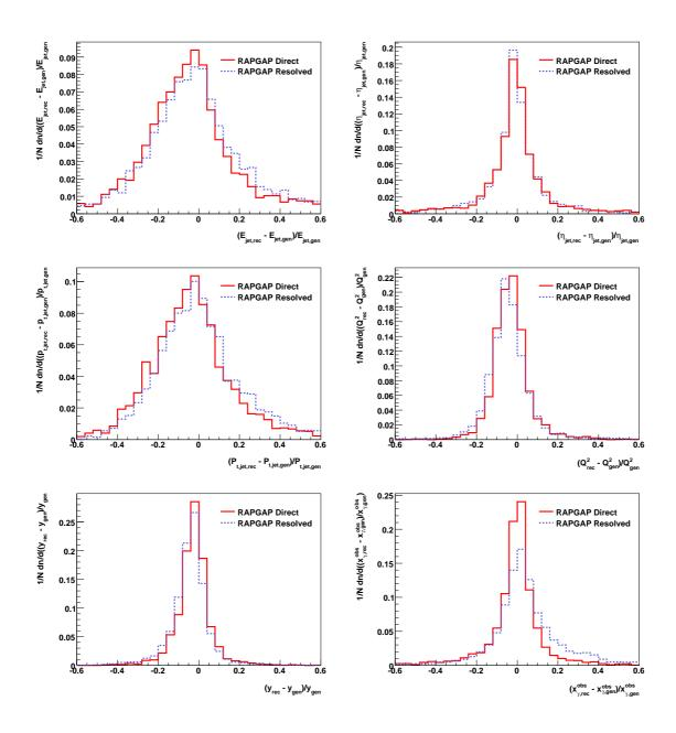
Figure 6.8: Relative resolution for DIS events in the jet variables  $E_{jet}$ ,  $\eta_{jet}$  and  $p_{t,jet}$  and in the event variables  $Q^2$ , y and  $x_{\gamma}^{obs}$ . The distributions are simulated separately for direct and resolved events by the RapGap Monte Carlo. All distributions are normalised to unity.
