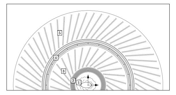
Figure 2.4: Radial view of the central tracking chambers of the H1 detector. From the innermost CST(1) going outwards the CIP(2), CJC1(3), COZ(4) and CJC2(5) are shown. The signal wires in CJC1 and CJC2 are aligned in beam direction and depicted as dots.
