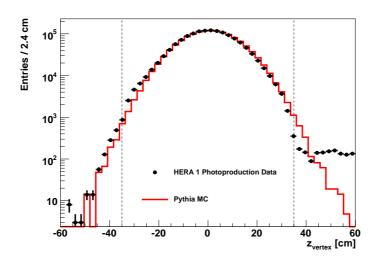
Figure 5.3: Distribution of the z-coordinate of the reconstructed primary vertex for photoproduction data. Also shown is the Monte Carlo distribution of signal events. The dashed lines indicate the cut at  $|z_{vertex}| < 35$  cm.
