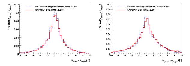
Figure 6.31: Resolutions of the polar angle  $\theta$  and the azimuthal angle  $\phi$  of the analysed jet. The resolutions are computed separately for photoproduction using the Pythia Monte Carlo and for DIS using the RapGap Monte Carlo simulation.
