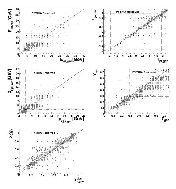
Figure 6.4: Reconstructed against generated variables for resolved photoproduction events as simulated by the Pyhia Monte Carlo. The index 'jet' denotes the analysed jet. The dashed lines indicate the applied cuts. The solid line serves as a reference to guide the eye.
