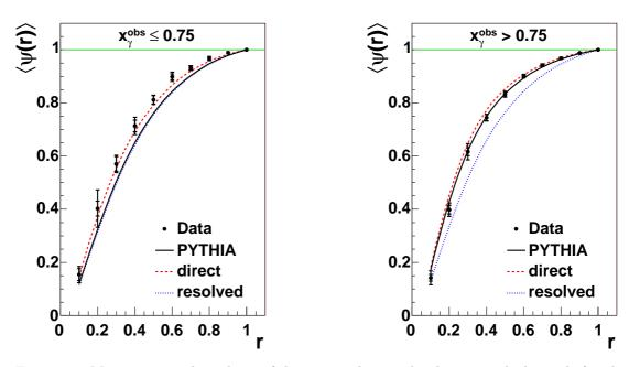
Figure 3.6: Mean integrated jet shape of the untagged jet in the charm-enriched sample for photoproduction. Shown are two different  $x_{\gamma}^{obs}$  regions and the total Pythia Monte Carlo prediction as well as separate direct and resolved expectations.
