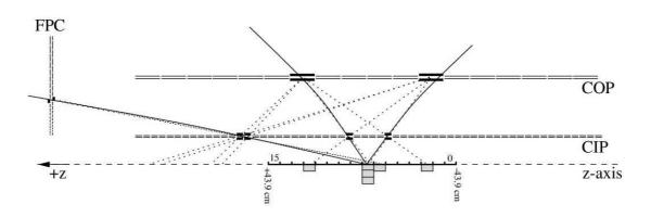
Figure 5.2: The z-vertex trigger: Particle trajectories (full lines) cause hits in the double layers of CIP, COP and FPC. Rays through the pads (dotted lines) are extrapolated to the z-axis. Only rays from particle trajectories form a significant peak in the z-vertex histogram.
