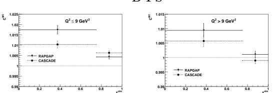
Figure 6.39: Comparison of the detector correction factors calculated by the RapGap and Cascade Monte Carlo simulations in DIS for the mean integrated jet shape  $\langle \psi(r=0.6) \rangle$ . The comparison is performed as a function of the variables  $x_{\gamma}^{obs}$  in two regions of  $Q^2$ . The error bars represent the statistical uncertainty of the Monte Carlo simulation.
