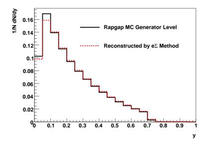
Figure 4.5: Distribution of the inelasticity in DIS on generator level and reconstructed by the  $e\Sigma$  method. The polar angle  $\theta_{e'}$  of the scattered electron in the Monte Carlo sample is limited to the backward calorimeter region causing a slump at y = 0.7 due to the geometrical acceptance of the calorimeter.
