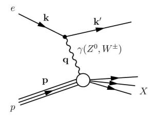
Figure 1.1: Schematical diagram of *ep* scattering including particle momenta.
