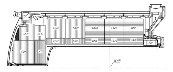
Figure 2.5: Side view of the liquid argon calorimeter. Visible is the separation into particular wheels. 'E' denotes the electromagnetic, 'H' the hadronic sections.
