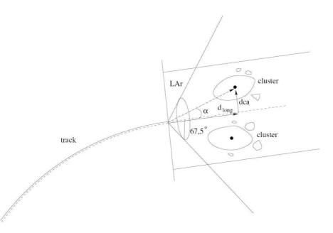
Figure 4.1: Scematic of the combination algorithm. The axis of the cone as well as the cylinder is a straight line extrapolation of the particle trajectory into the calorimeter. The distance of closest approach dca of a cluster is defined with respect to this line. This figure was taken from [76].
