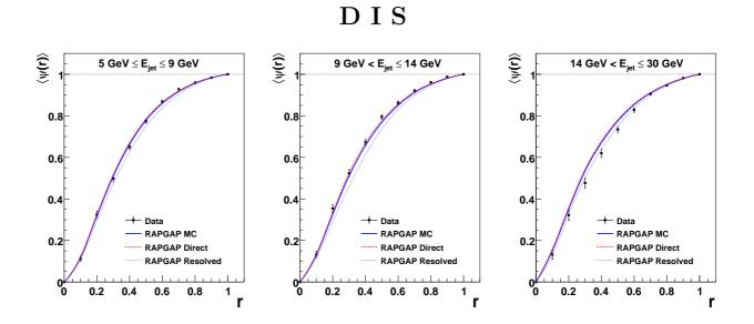
Figure 6.20: Mean integrated jet shape  $\langle \psi(r) \rangle$  in DIS at detector level as function of the cone radius r for three different regions of the jet energy  $E_{jet}$ . RapGap charm Monte Carlo prediction is shown together with separate direct and resolved expectations. Only statistical errors of the data are shown. The statistical errors of the Monte Carlo simulation are negligible.
