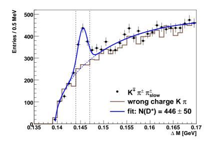
Figure 5.5: Distribution of the difference  $\Delta m$  between the invariant mass of the D<sup>\*</sup> candidate and the D<sup>0</sup> candidate after photoproduction jet selection for the ET33 sample. The dotted lines indicate the signal region.
