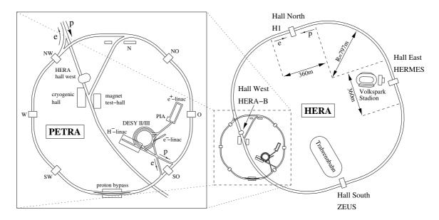
Figure 2.1: The HERA collider and its pre-accelerators.
