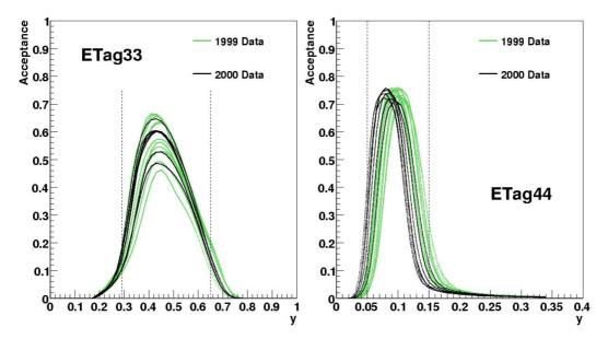
Figure 5.4: Acceptance of the ET33 (left) and ET44 (right) as function of the inelasticity y. The parametrisations also include inefficiencies due to the trigger requirements and due to cuts on the position of the energy deposition of the scattered electron within the tagger. Each year is subdivided into several periods during which the acceptance was constant. The vertical lines indicate the selected y-region to achieve acceptances of higher than 10%.
