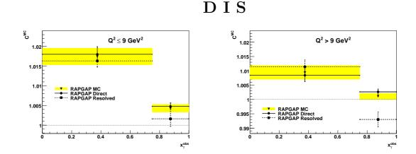
Figure 6.30: Detector correction factors for the mean integrated jet shape  $\langle \psi(r = 0.6) \rangle$  in DIS as a function of the variable  $x_{\gamma}^{obs}$  in two regions of  $Q^2$ , determined using the RapGap Monte Carlo simulation. The factors are shown for the total Monte Carlo and separately for direct and resolved processes. The error band and bars represent the statistical uncertainty of the Monte Carlo simulation.
