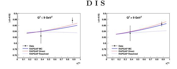
Figure 6.25: Distributions of the mean integrated jet shape at fixed value r = 0.6 at detector level as function of  $x_{\gamma}^{obs}$  in two regions of  $Q^2$ . RapGap charm Monte Carlo prediction is shown together with separate direct and resolved expectations. Only statistical errors of the data are shown. The statistical errors of the Monte Carlo simulation are negligible.
