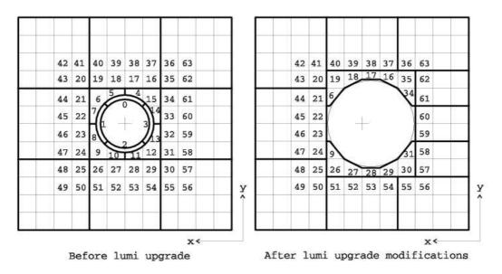
Figure 2.7: The cells of the inner region of the SpaCal before and after reconstruction due to the luminosity upgrade including their numbering. The origin of the coordinate system is illustrated by a cross within the central region.
