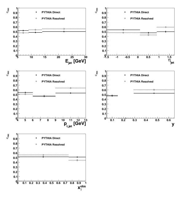
Figure 6.1: Reconstruction efficiency for direct and resolved photoproduction events as function of the variables E,  $\eta$  and  $p_t$  of the analysed jet as well as y and  $x_{\gamma}^{obs}$ . The efficiencies are calculated with the Pythia Monte Carlo simulation.
