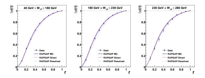
Figure 6.21: Mean integrated jet shape  $\langle \psi(r) \rangle$  in DIS at detector level as function of the cone radius r for three different regions of  $W_{\gamma p}$ . RapGap charm Monte Carlo prediction is shown together with separate direct and resolved expectations. Only statistical errors of the data are shown. The statistical errors of the Monte Carlo simulation are negligible.
