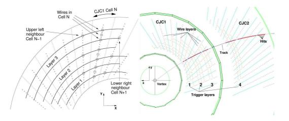
Figure 5.7: Radial view of the CJC. The left drawing shows the division into trigger cells and the wires from neigbouring cells taken into account for reconstruction of track segments. The right drawing gives an overview of both CJCs and the  $4 \times 3$  wire layers used by the FTT.
