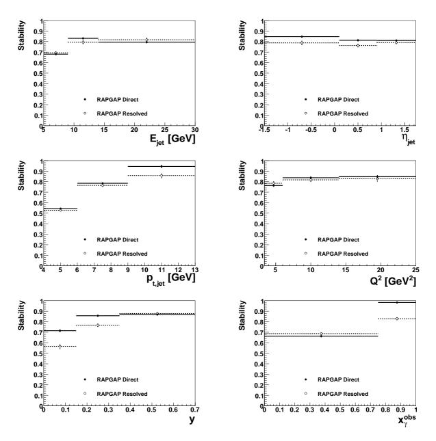
Figure 6.12: Stabilities of DIS events in the jet variables  $E_{jet}$ ,  $\eta_{jet}$  and  $p_{t,jet}$  and in the event variables  $Q^2$ , y and  $x_{\gamma}^{obs}$ . The stabilities are calculated separately for direct and resolved events by the RapGap Monte Carlo.
