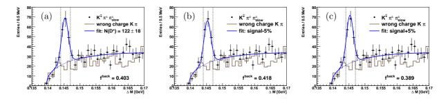
Figure 6.33:  $\Delta m$  distribution of the ET44 selection in photoproduction including the fit describing signal and background (a). The function describing the signal is scaled down by 5% in (b) and up by 5% in (c). Also displayed is  $f^{back}$ , the fraction of background events in the  $\Delta m$  signal region between the dashed lines as obtained by the fits. The function describing the background is not subject to the variation.
