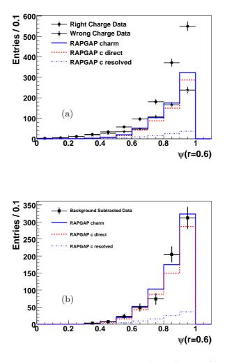
Figure 6.13: Integrated jet shape of the right charge ( $\psi^{\text{meas}}(r = 0.6)$ ) and wrong charge data ( $\psi^{\text{back}}(r = 0.6)$ ) together with the total RapGap charm Monte Carlo and its direct and resolved components on detector level (a). The Monte Carlo distribution is normalised to the integrated lumonisity of the data. In (b) the background subtracted data ( $\psi^{\text{sig}}(r = 0.6)$ ) is shown with the same Monte Carlo.
