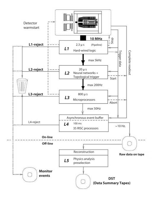
Figure 4.5: The H1 trigger system.
