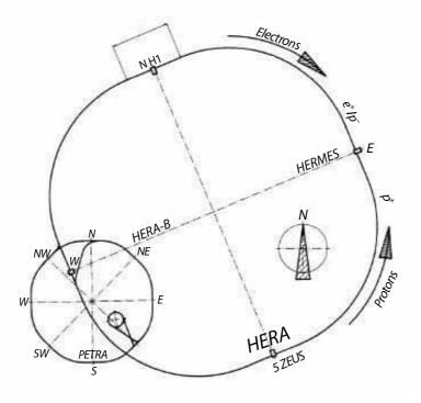
Figure 3.1: Schematic view of the HERA collider ring.
