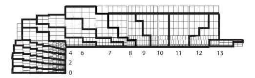
Figure 4.6: The projective Big Towers in LAr calorimeter. Each tower points toward the nominal interaction point.
