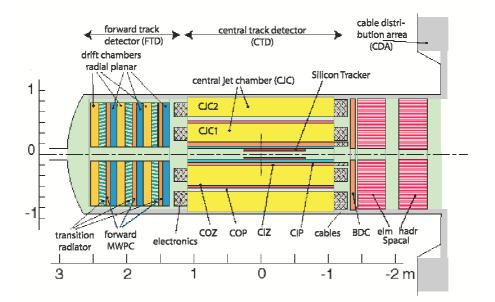
Figure 4.3: The side view of the H1 tracking system.
