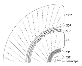
Figure 4.4: The central tracking detectors.
