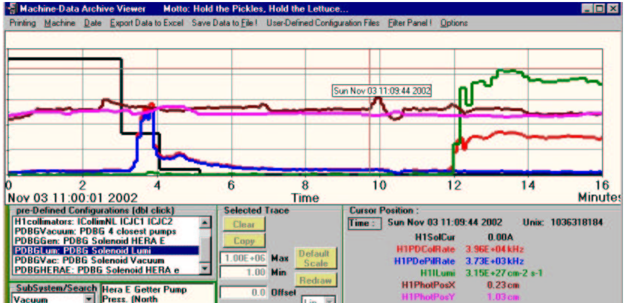
Figure 43: Shown as a function of time are: black stepped line, the current in the H1 solenoid (only values of current at which sampling occurred shown); blue line which peaks at 3.5 mins, rate of positron beam-gas induced Bethe-Heitler events; central dark red and pink lines, the x and y positions of the photons impacting on the photon detector of the luminosity system; green line that rises to become that highest in the plot at 12 mins, the measured luminosity; red line that rises to a central position at 12 mins, the rate measured in the luminosity system's photon detector.
