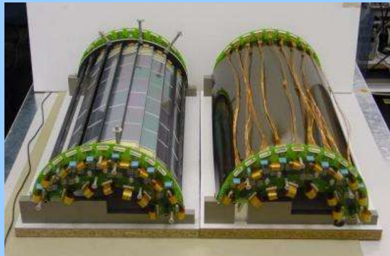
Both halves assembled; on right: power cables from back to front
