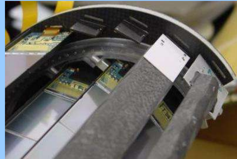
During assembly, dummy »ladders« are replaced by the real ones
