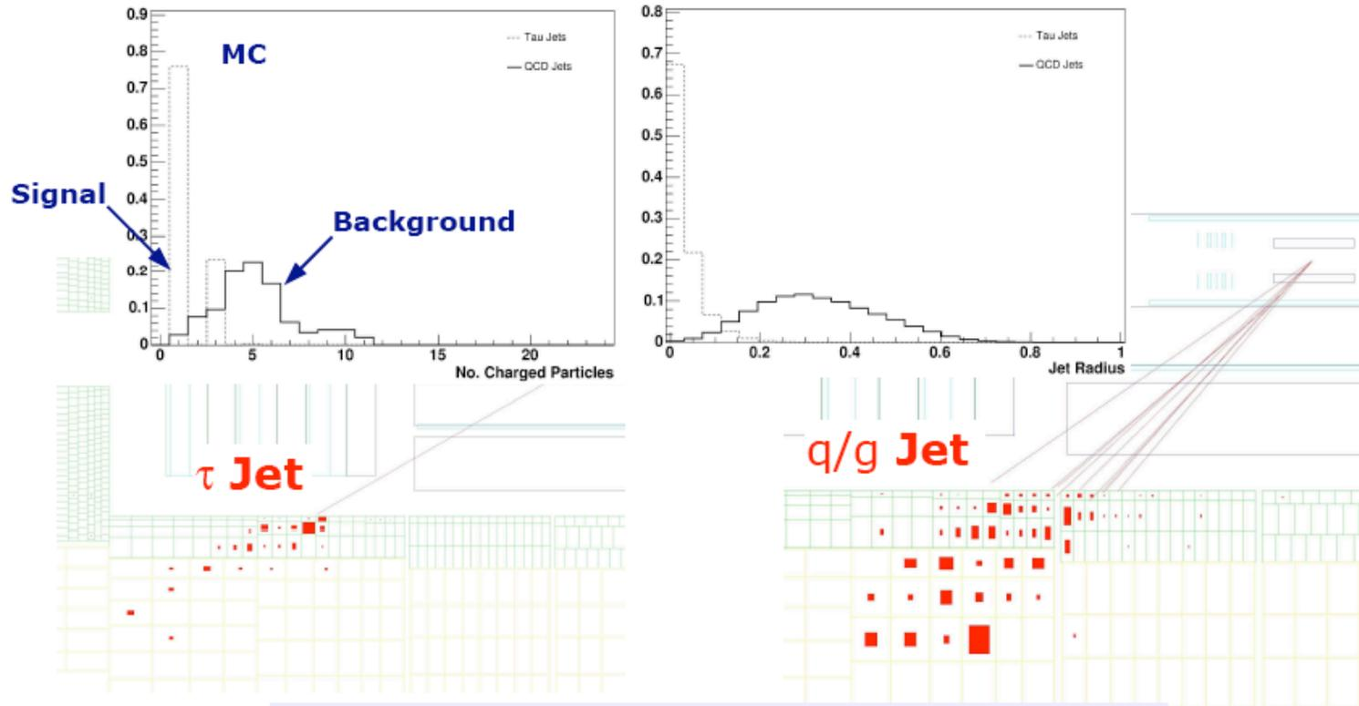
A hadronic  $\tau$  decay originates a jet with very specific characteristics : **collimated energy deposits in Calorimeter** and **few charged particles in Tracking detectors**
