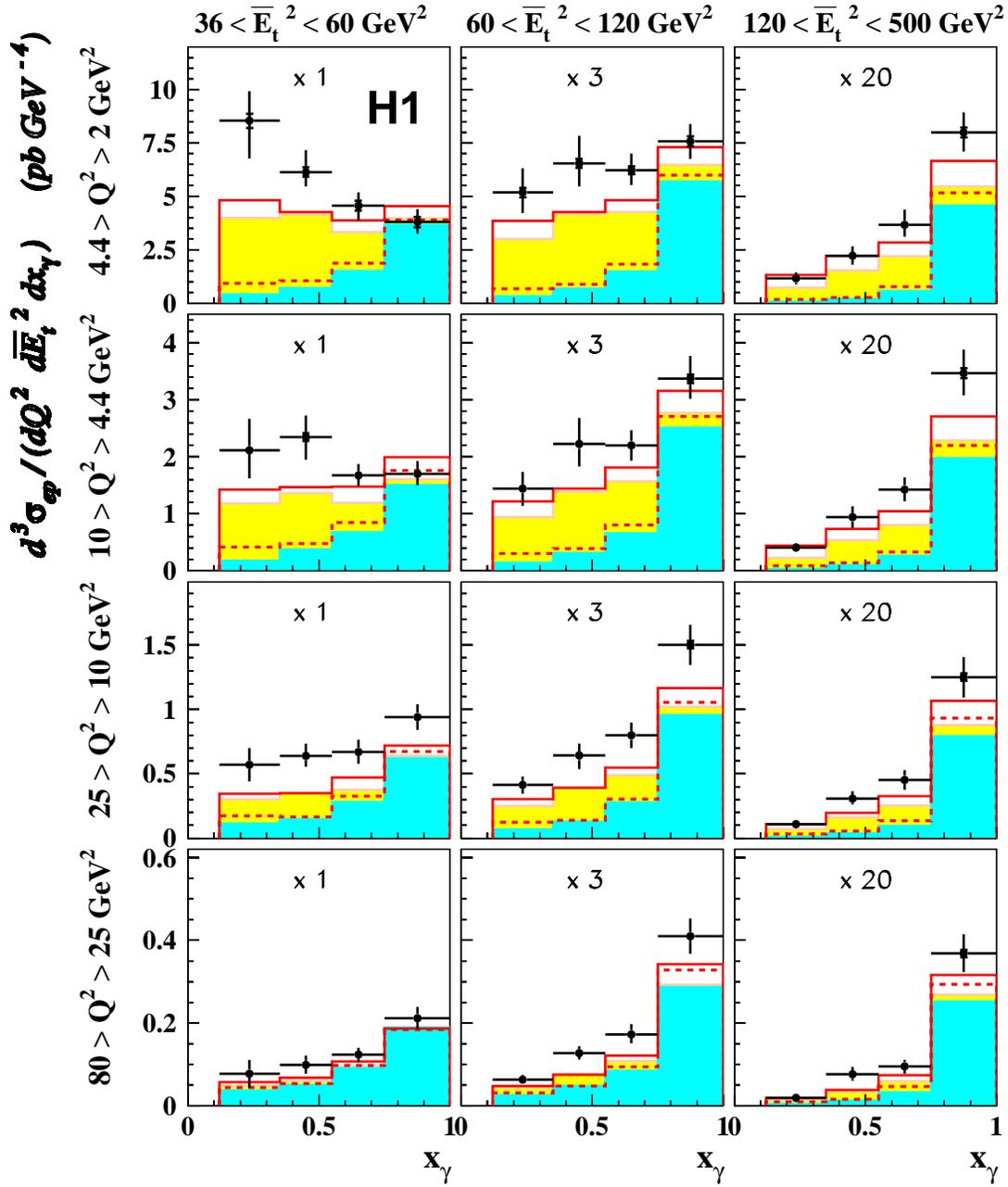
Figure 3: Triple differential dijet cross-section as a function of  $x_\gamma$ ,  $\overline{E}_t^2$  and  $Q^2$ . The data are compared to HERWIG and RAPGAP MC predictions. Separately shown are the direct (dir) and the resolved component of transversally polarized  $\gamma$  (res<sub>T</sub>).
