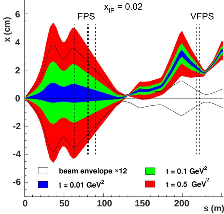
Figure 2: Beam envelope [2] as a function of the distance  $s$  to the H1 vertex in the  $x$  projection, for the  $p$  beam and diffractive protons at  $x_{IP} = 0.02$  and  $|t| = 0.01, 0.1$  and  $0.5 \text{ GeV}^2$ . The locations of FPS/VFPS stations are indicated by the vertical lines.
