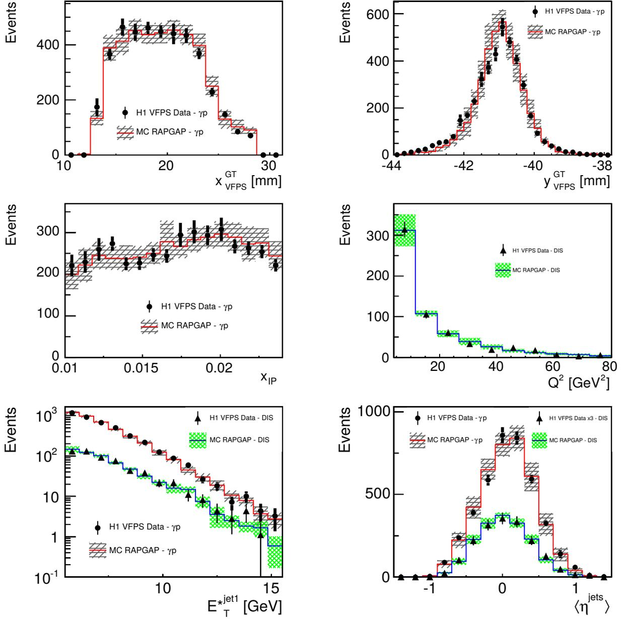
Figure 3: Comparison of the photoproduction data (dots) and DIS data (triangles) with the reweighted RAPGAP MC simulation (solid line) as a function of coordinates  $x$  and  $y$  in VFPS,  $x_P$ ,  $Q^2$ ,  $E_T^{*jet1}$  and  $\langle \eta^{jets} \rangle$ . The systematic uncertainties are shown as bands on the histograms. For better visibility the  $\langle \eta^{jets} \rangle$  DIS distribution is multiplied by a factor 3.
